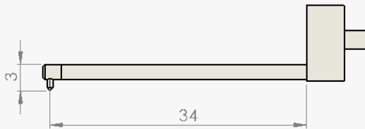
Probe arm \varnothing 4.5mm (Cod. M1AAMA)
